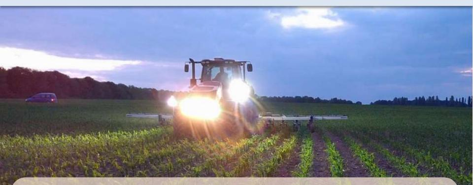
OPTIONAL: special headlight for symmetrical and uniform illumination with cable and mount allows the cultivator to work at night.
