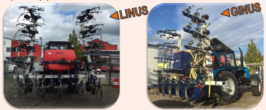
The GELIO cultivator can optionally be equipped with the LINUS system for input of liquid fractions in the inter-row or in the row, as well as on the leaf surface. The system GINUS can be used for input of granular fertilizers in the inter-row or under the sweeps during the cultivating.
