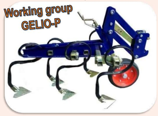
Working group GELIO-P: there are 5 S-spring tines with 150 mm sweeps in this working group. It is possible to use this working group universally for all kinds of crops, if you remove 2 S-Spring tines and adjust the row distance.
